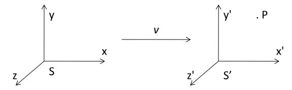
The frame S' moves with velocity v relative to the frame S along x axis. According to the Galilean transformation (non relativistic), we have for any point P:
