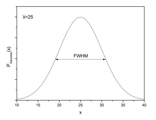
Full width at half maximum = FWHM =  $2\sqrt{2\ln 2\sigma} = 2.355\sigma$  with  $\sigma = \sqrt{\overline{x}}$
